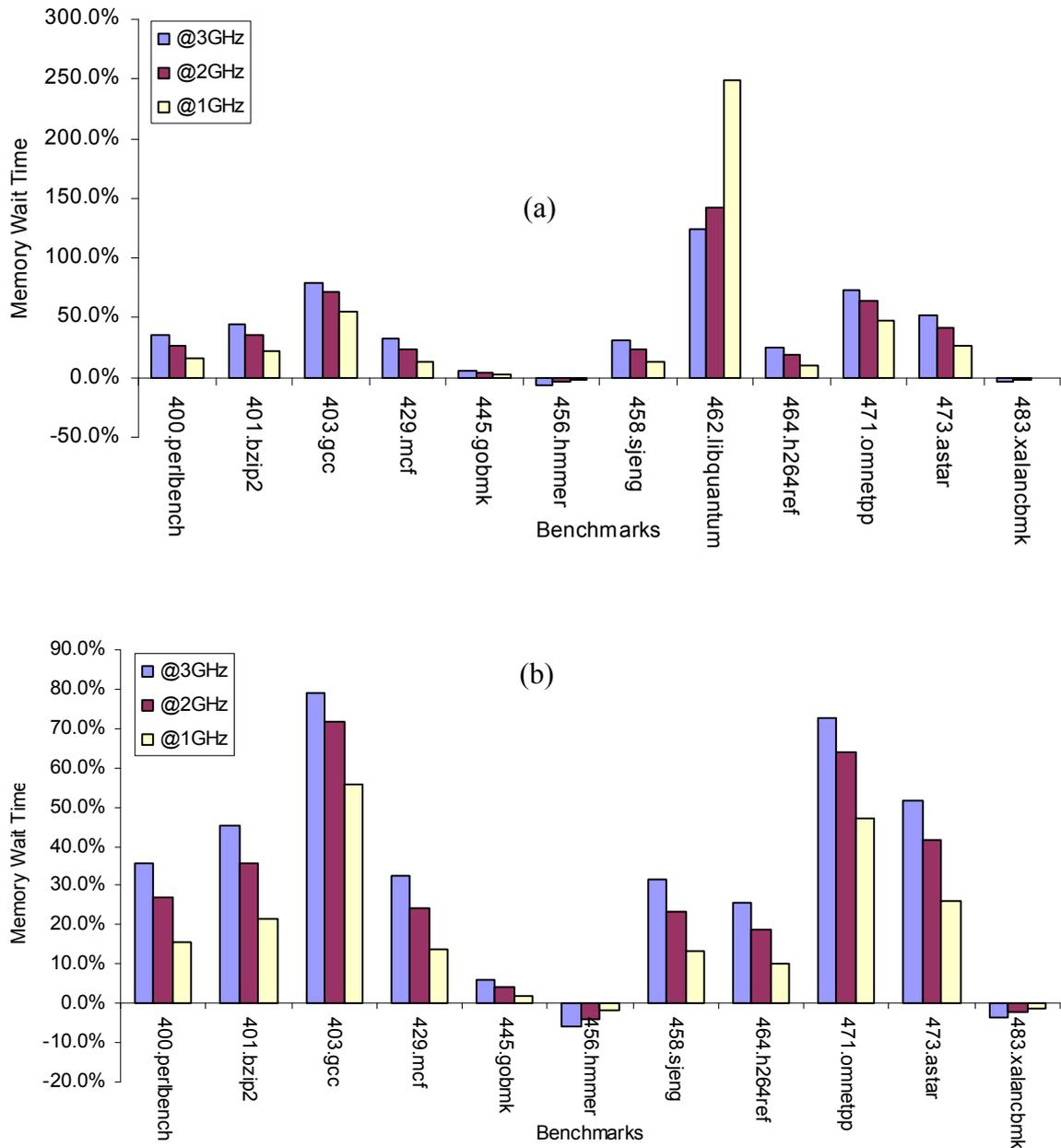
Figure 4: (a) The comparison of normalized task completion time @1GHz, @2GHz and @3GHz processor frequency on AMD processors, (b) Magnified view of (a) without 462.libquantum benchmark.
