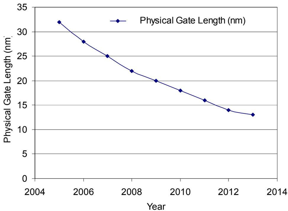
Figure 2: Scaling of successive MPU Physical Gate length from ITRS in near future
