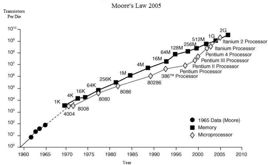
Figure 1: Scaling of transistors, the number of transistors is expected to continue to double about every two years, in accordance with Moore's Law. Over time, the number of additional transistors will allow designers to increase the number of cores per chip.
