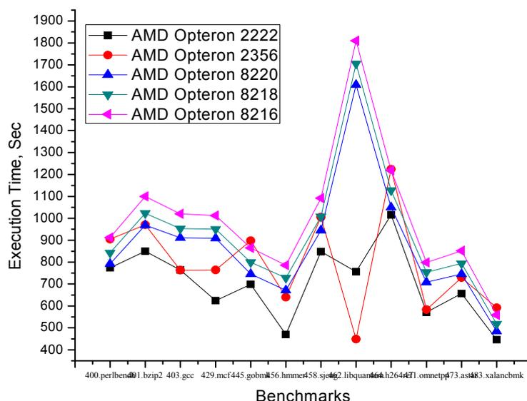
Figure 3: Execution Time variation with Benchmarks in different AMD Opteron Series Processors
