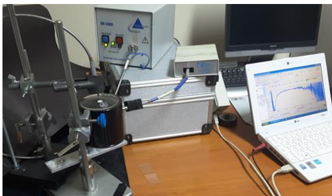
Fig.1. The Ocean Optics micro - spectrometer
